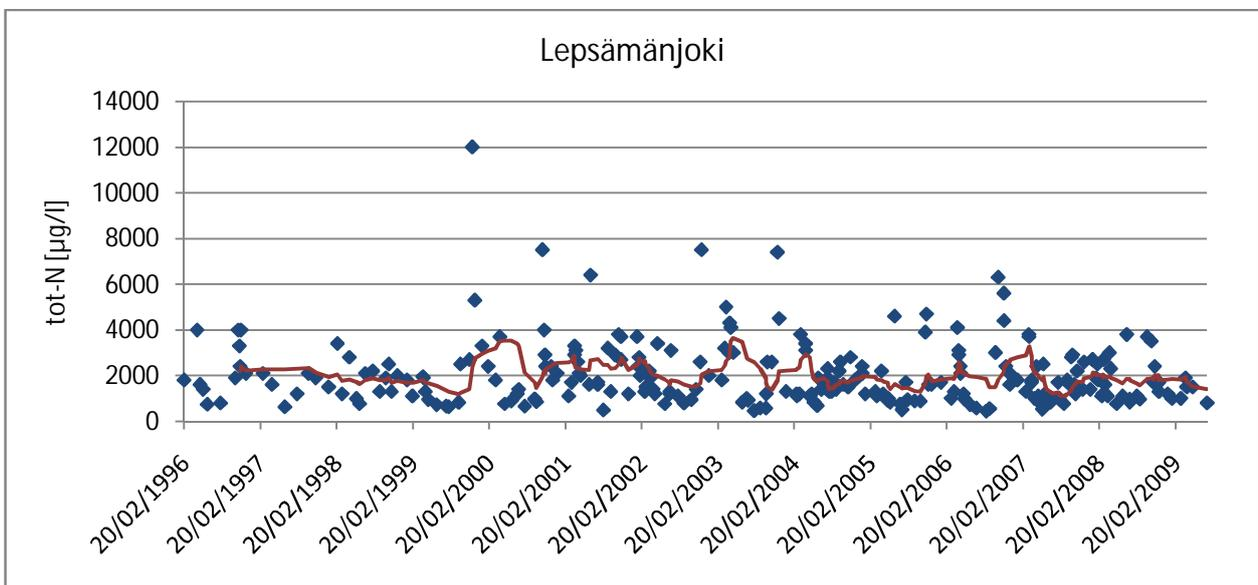
Figure 7. Observed total nitrogen concentrations at the outlet of the river Lepsämänjoki. Red line is the moving average of the concentrations. Katri Rankinen / SYKE
